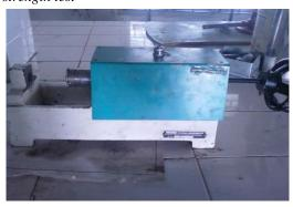
The procedure to extract the shear strength of sand is as same as compression strength. This is accomplished by changing the load surface on the testing machine from compression pads to shear pads. The specimen then rupture's in shear along its longitudinal axis, when sufficiently loaded. Shear strength may vary from 10 to 50 KPa.
