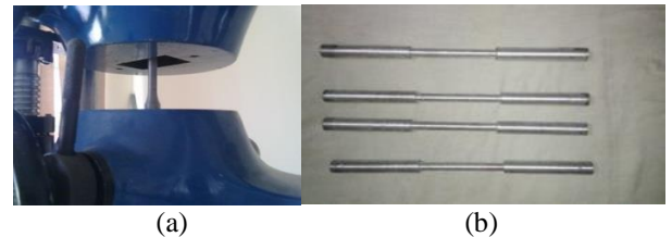
Fig. 1. (a) UTM machine showing sample specimen of A1100 tested for tensile and ductility. (b) Specimen of alloy A1100 before mechanical test on UTM.
