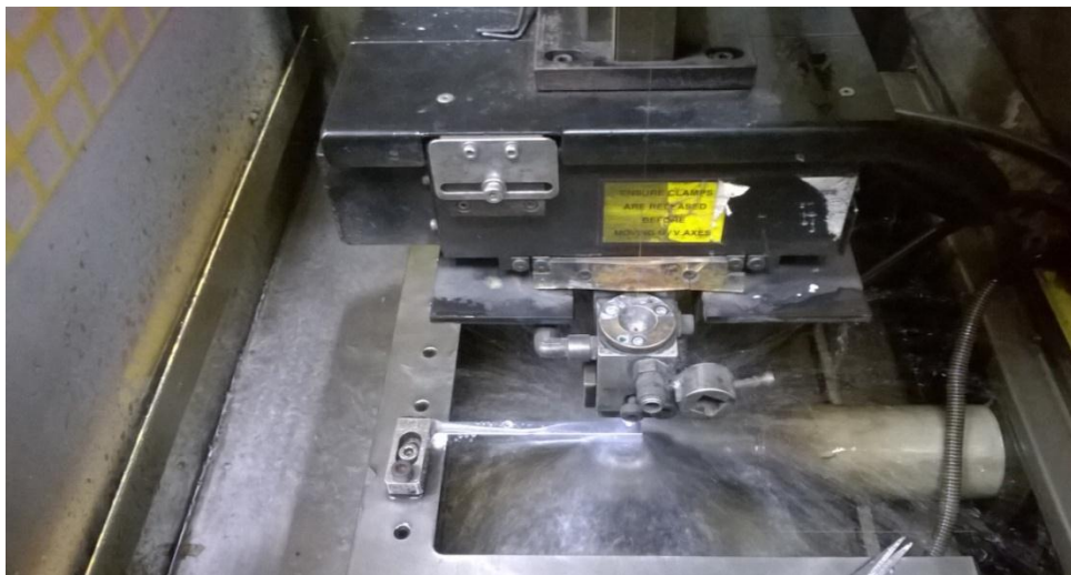
Fig. 2: Image of Wire EDM during machining (Model: Electronica Eco cut machine)
