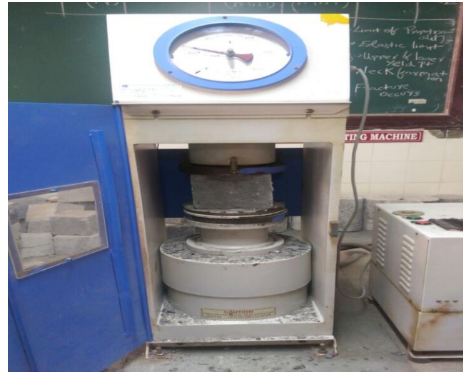
Figure :2 Compressive Strength Test Set up
