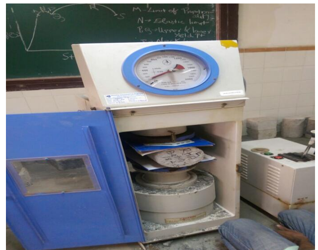
Figure :3 Split Tensile Strength Test Set up
