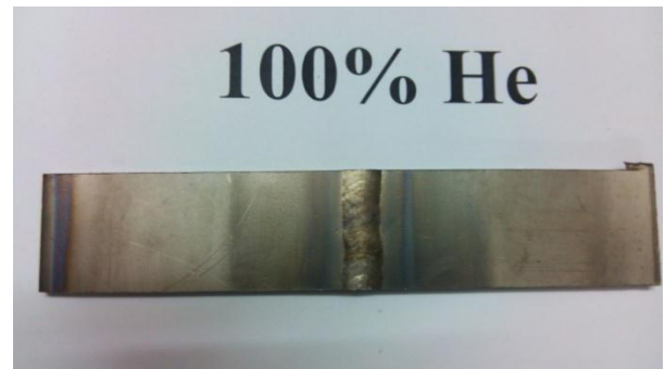
Fig 4.5 welded job for making tensile test specimen, when 100% He used as a shielding gas.
