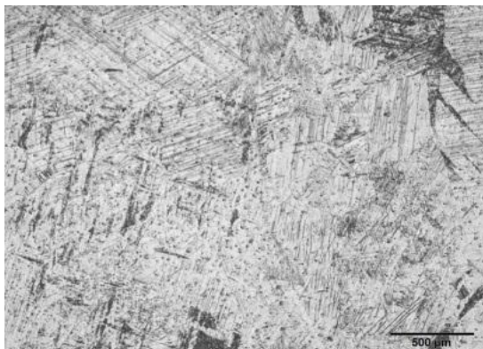
Fig 4.7 weld metal microstructure of pure titanium grade 2 with 100% Ar as shielding gas.
