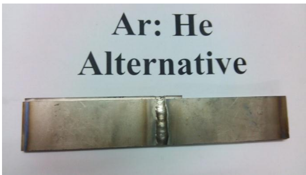
Fig 4.2 welded job for making tensile test specimen, when alt gases used as a shielding gas.
