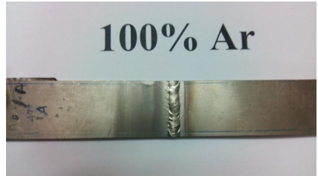
Fig 4.4 welded job for making tensile test specimen, when 100% Ar used as a shielding gas.
