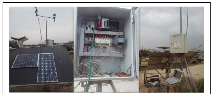
Fig.5. NOCT setup with data logging and test specified module placed
