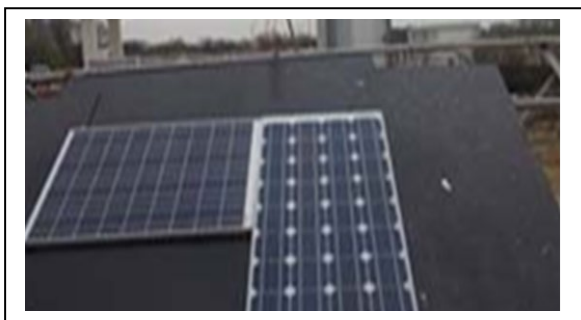
Fig.3. Placement of both Technology models at NOCT Test Bed Setup
