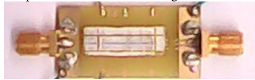
Fig. 4. RF MEMS die attach with wire bonding
