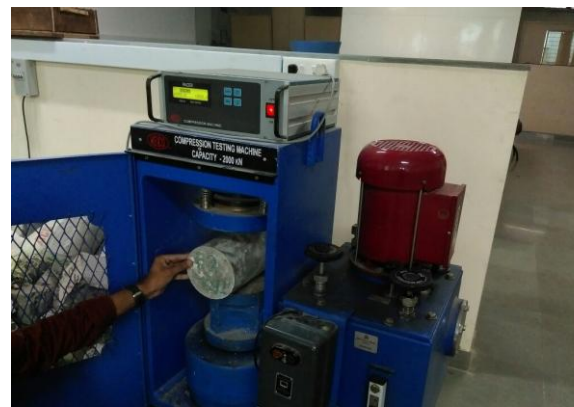
Figure 2: Splitting Tensile Strength Test Set up
