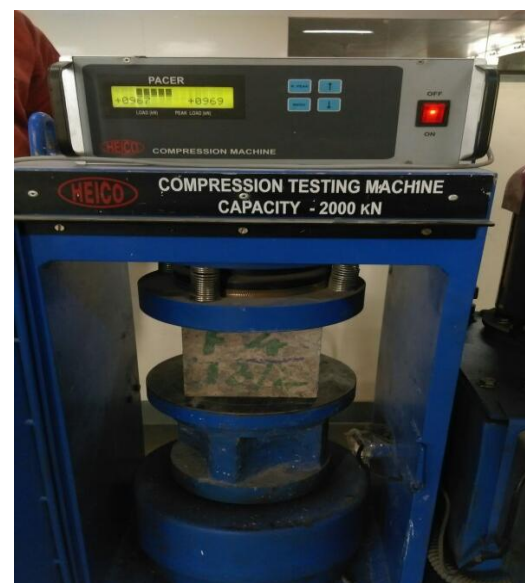
Figure 1: Compressive Strength Test Set up.
