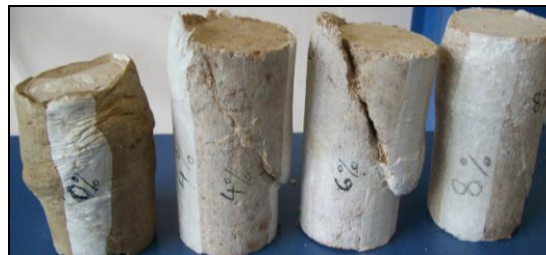
Figure 3: Triaxial compression (CU) samples after test
