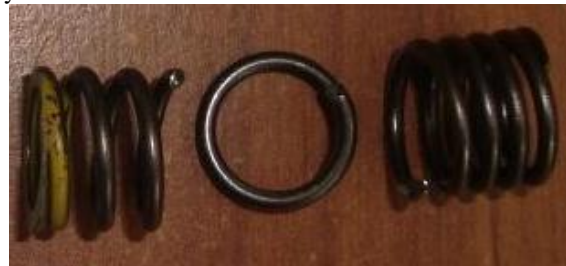
Fig 3 As received photograph of failed spring
