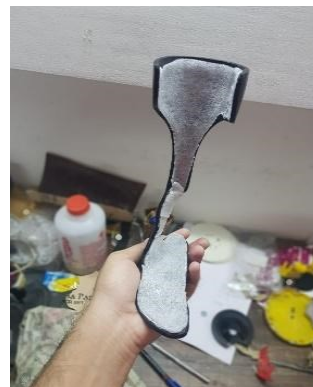
FIGURE 10- Cushioning done on manufactured new AFO
