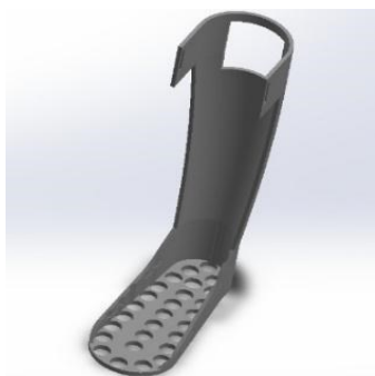
FIGURE 6- AFO model after topology mass optimization.
