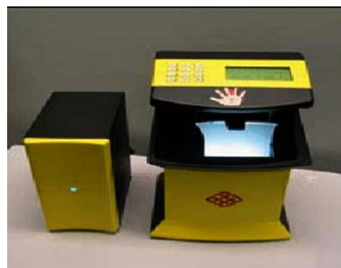
Figure 2: The outlook of developed Palmprint acquisition device [10]
