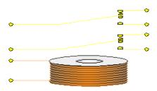
This relay is a Double Pole Double Throw relay. It operates like the SPDT relay but has twice as many contacts. There are two completely isolated sets of contacts.
