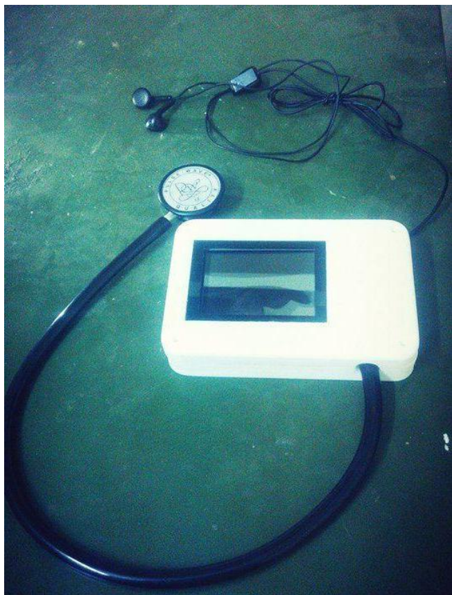
Figure 2: Image showing the outer appearance of the device. Sound inputs are taken with the stethoscope diaphragm and any earphone can be connected for getting clean and amplified sound output.
