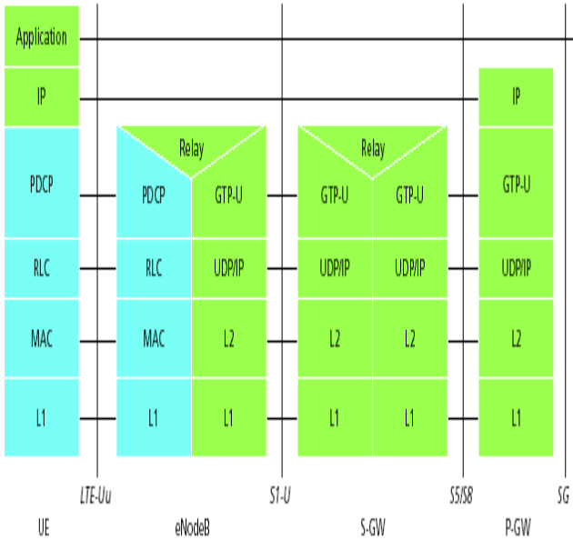
Fig. 6. The LTE User Plane Protocol Stack.
