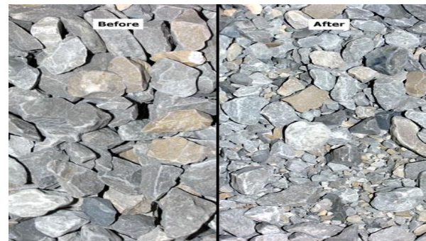
Figure 3: Breakage of aggregate samples after soundness test
