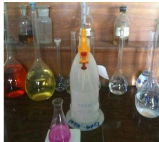
Figure 4: Chemical method for alkali silica reaction
