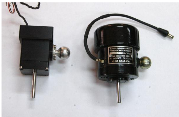
BLDC Motor Existing wound field DC motor
