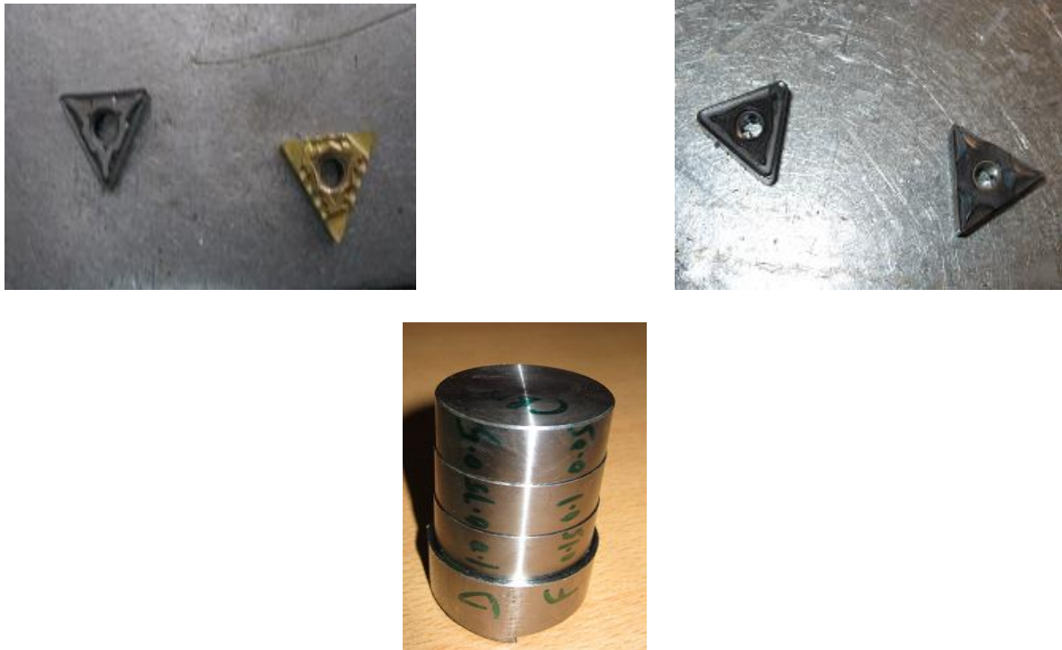
Figure 4.1 Cutting Inserts and Workpiece Material
