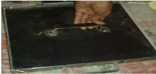
Figure.3, Flat mould for face sheets preparation.
