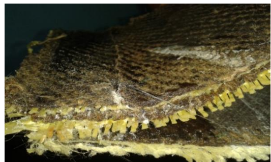
Fig.13, delaminating and debonding at an edge of core Afterprocess.
