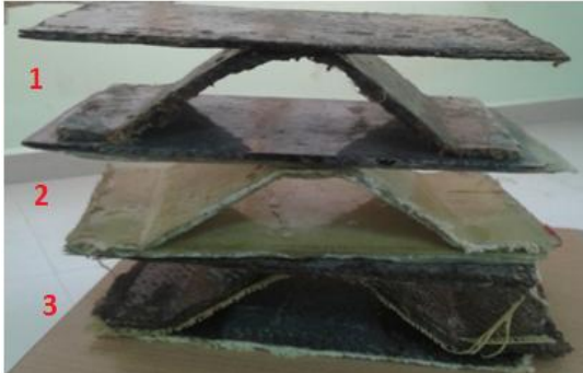
Figure. 6, Final hybrid composite corrugated sandwich coupons.
