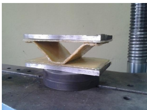
Figure. 7, Experimental set up for hybrid composite coupons under Universal Testing Machine.
