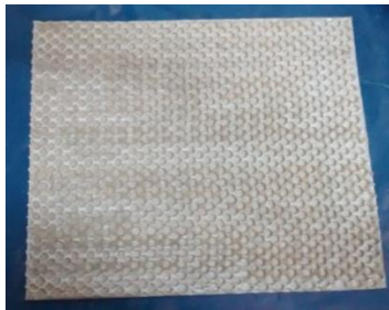
Fig.1: Prepared Glass Fiber Honeycomb Core
