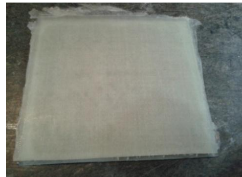
Fig.3. Prepared Honeycomb Sandwich (Honeycomb Core between 2 Face sheets)
