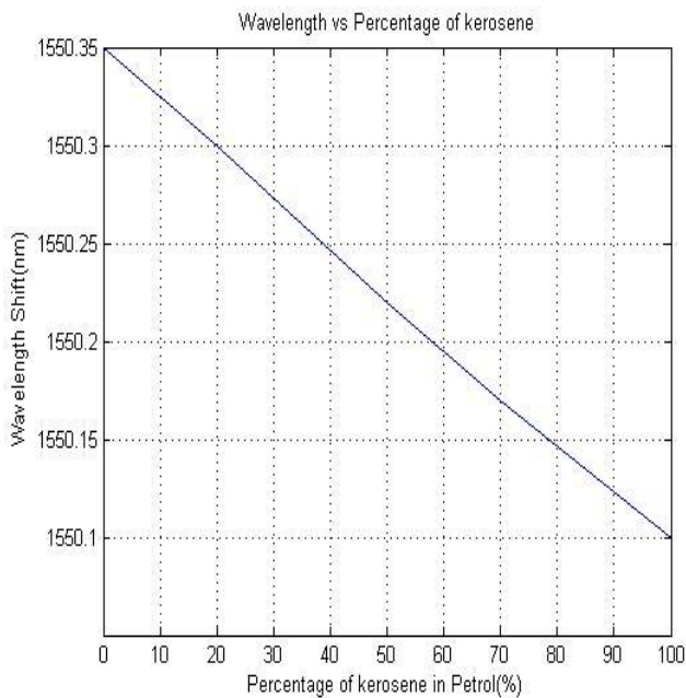
Fig 3: Change in wavelength shift with percentage of kerosene added.
