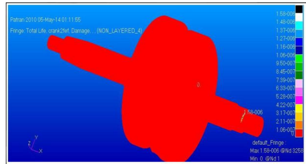
Fig. 7. Critical locations for damages of crankshaft
