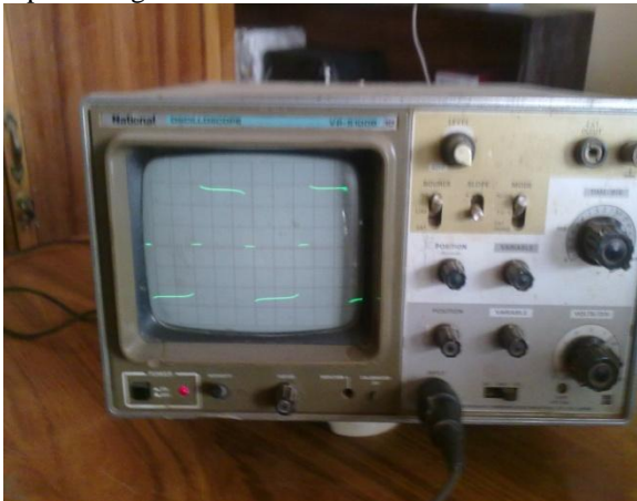
Figure 7: Inverter output wave on oscilloscope
