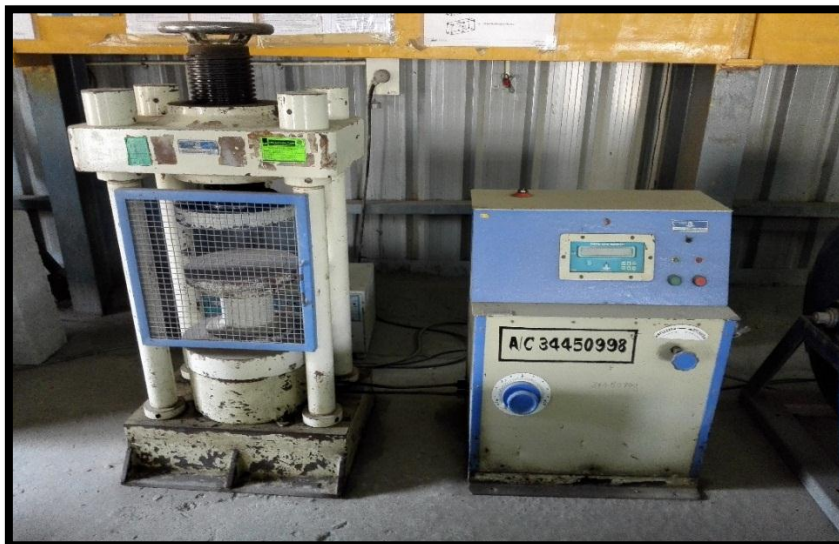
Fig-2: Experimental Setup for Compressive test
