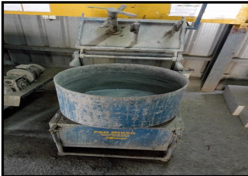
Fig-1: Pan Mixer (Experimental Setup for Concrete Mixing)
