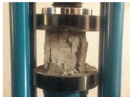
Fig. 7 Behavior of Control Specimen
