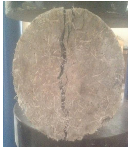
Fig. 5 Fibers Stretched in Split Tensile Test
