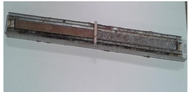
Fig. 3 Specimens curing process in the channel
