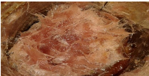
Fig. 1 Mixture of glass fiber and resin
