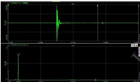
Fig. 7 (a) Free vibration experimentation test for the Specimen1
