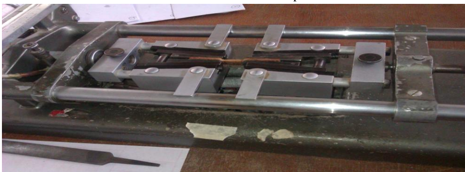
Plate 1. Tensile test experiment using tensometer equipment
