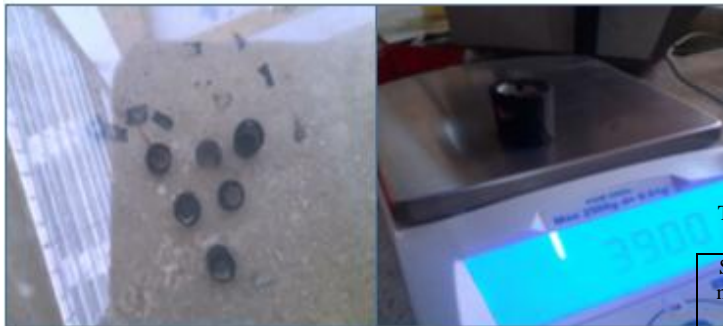
Figure 3(b): Samples under curing and reweighing process
