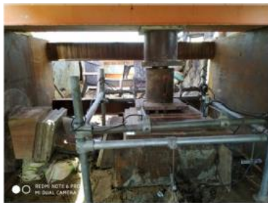
Testing on concrete to rock interface
