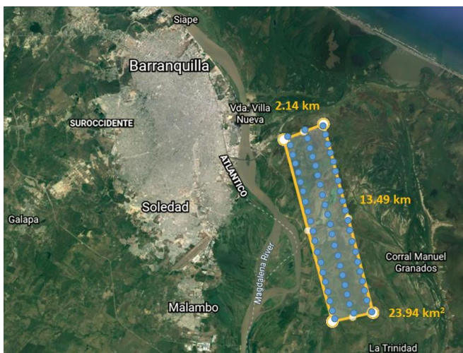
Fig. 6. The layout of the potential wind farm
