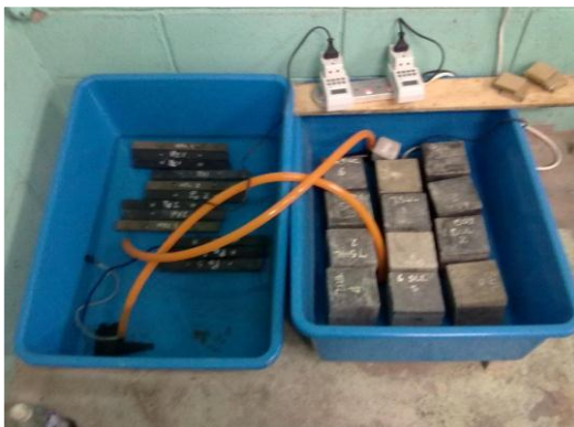
Fig 1. Specimen in sulphate solution with alternate wet and dry cycle arrangement.
