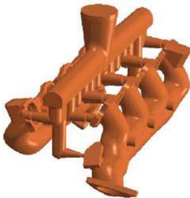
Fig(3.1) Mould tree assembly
