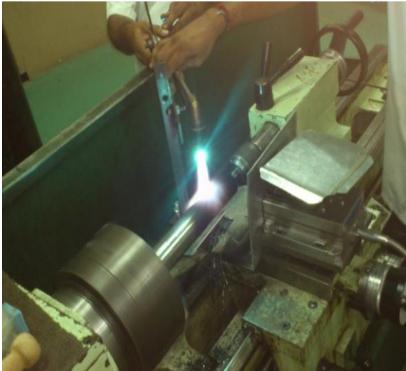
Figure3: Heating of the Die steel using oxy-acetylene flame
