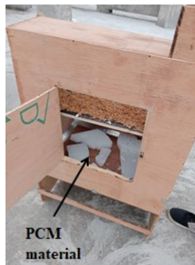
Fig 2 Photograph of Phase change material paraffin wax and paddy grains in solar air heater
