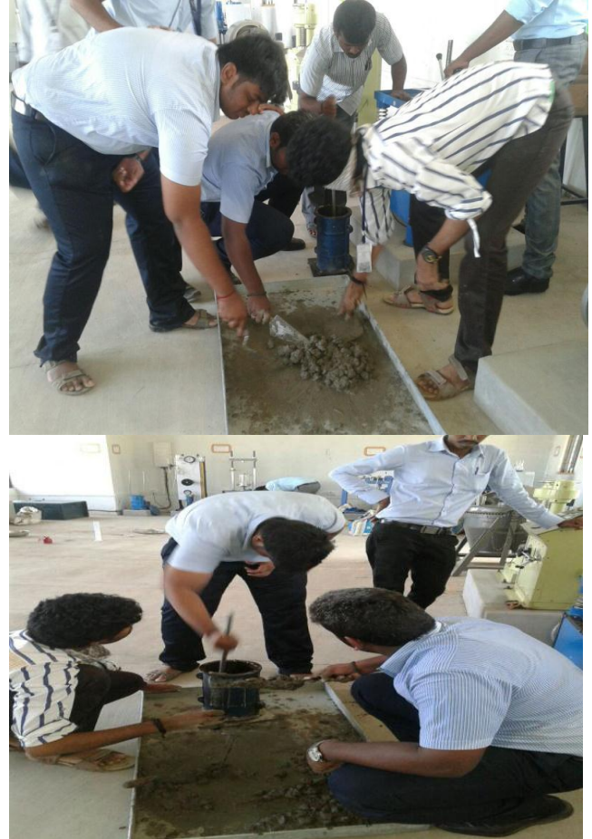
Fig 4: Casting Of Concrete
