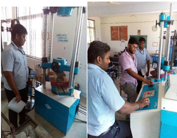
Fig 5: Split Tensile Strength Test In Utm
