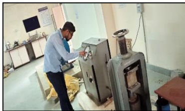
Fig.-4 Performing Compressive Strength Test
