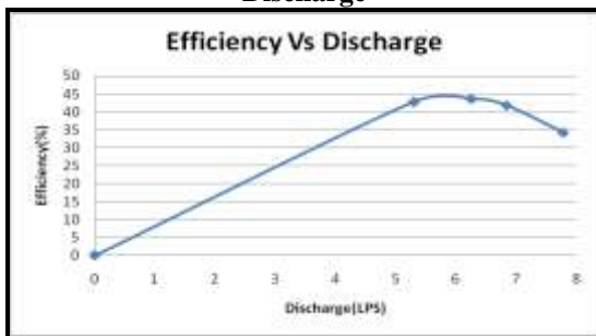
Fig.20: Graphically curve Efficiency vs Discharge
