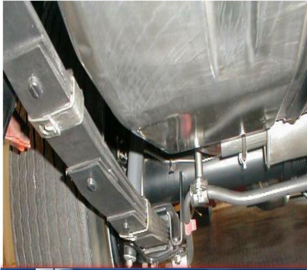
Figure A 1 traditional leaf spring arrangement
