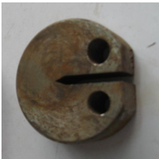
Figure 8 DC[T] Specimen 12mm thick having wire-cutting notch of an angle 38^{\circ} .
