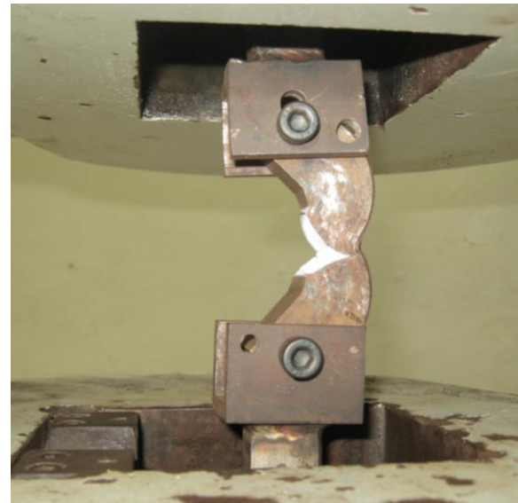
Figure 9. Experimental set-up showing crack propagation in loaded specimen
