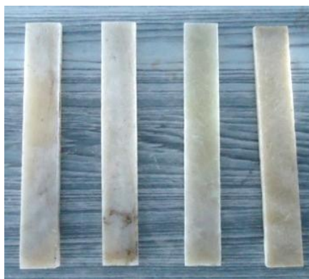
Fig. 2 Specimens of GFRP laminate with dimensions of 250 mm×30 mm×8 mm
