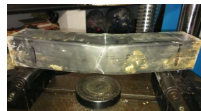
Figure 7- failure of composite beam section
