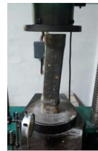
Figure 6- failure of composite section under compression
