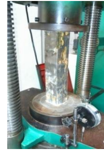
Figure 5- failure of composite section under compression
