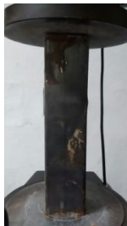
Figure 4- failure of composite section under compression
