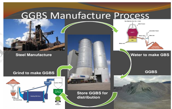
Fig 1.1 Manufacture of GGBS
