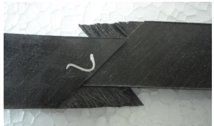
Fig-4: Specimen failure in in-plane shear
