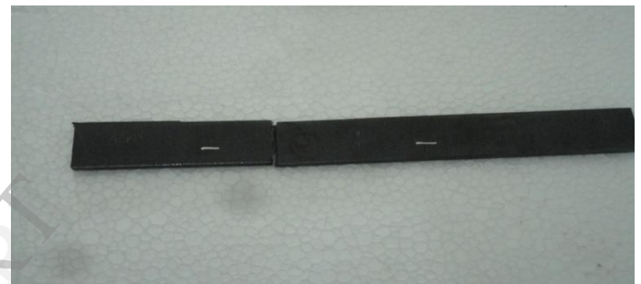
Fig-3: Specimen Failure in Transverse tensile loading
