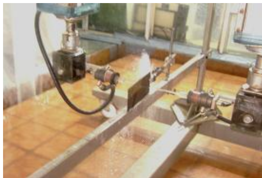
Fig.4 shows the 'C' Scan set up of cured laminate.
