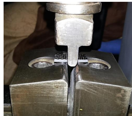
Fig. 6 Interlaminar Shear Strength test set up at UTM.
