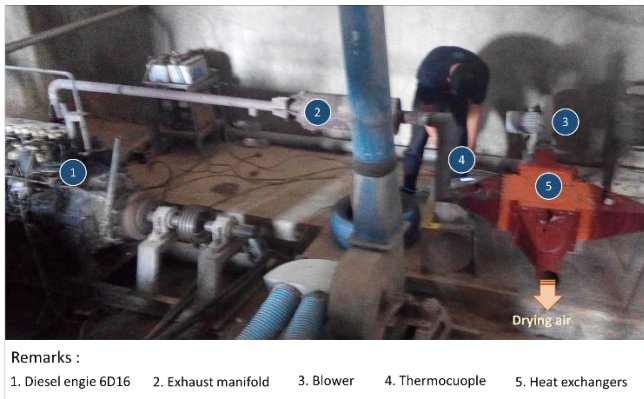
Figure 4. Experimental equipment of compact heat exchanger
