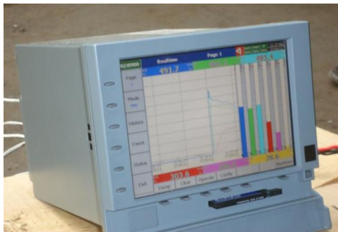
Plate 1. RD8900 Paperless Temperature Recorder rear and front view showing six channel displays
