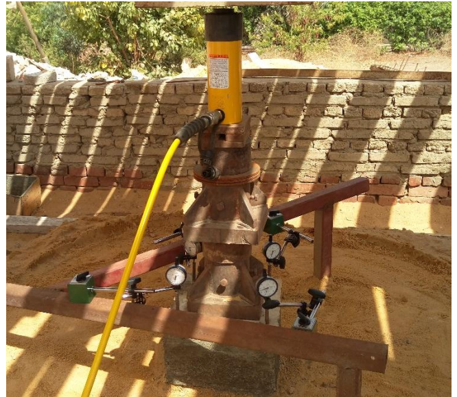
Fig. [14] Loading Jack and Dial Gauges Setup for Group (1) – Single Pile
