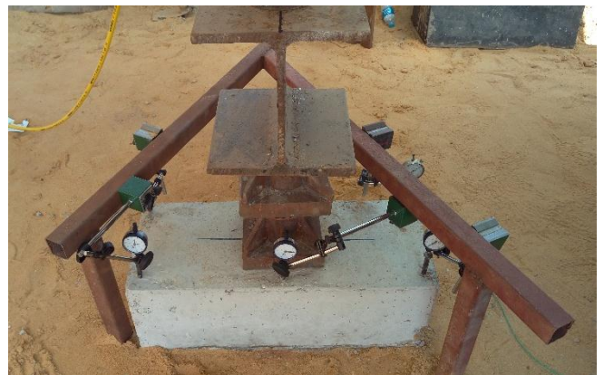
Fig. [15] Reference Beams and Dial Gauges Setup for Group (2) – Group of Two Piles
