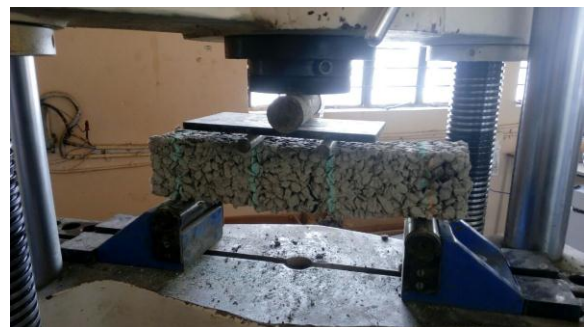
Figure No. 4: Flexural Strength Test
