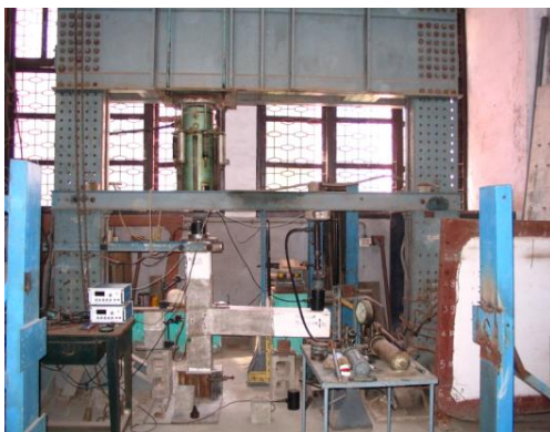
Fig. 16: Strengthened specimen for testing
