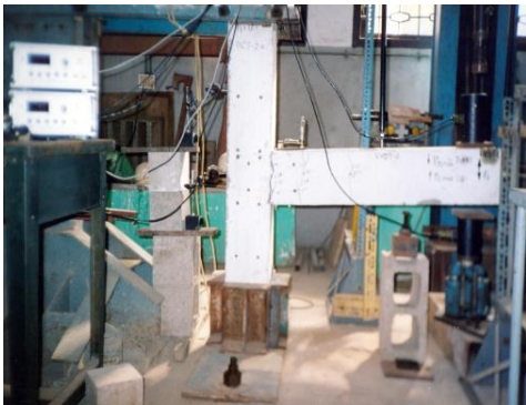
Fig. 9: Flexural failure of IS: 13920 specimens
