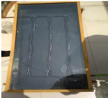
Plate 4 Twisted Tubes Experimental Set Up
